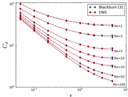
Figure 1: Comparison of peak coefficients of drag,  $C_d$ , for a stationary sphere in an oscillating flow.
