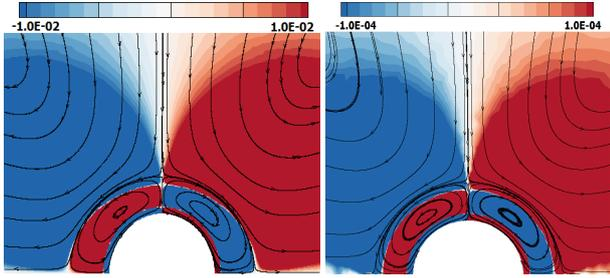
Figure 2: Flows generated using: (left) DNS for  $Re = 100$ , when  $\epsilon = 0.25$ , and (right) WNL for  $\Omega = 100$ . The colour contour represents vorticity.
