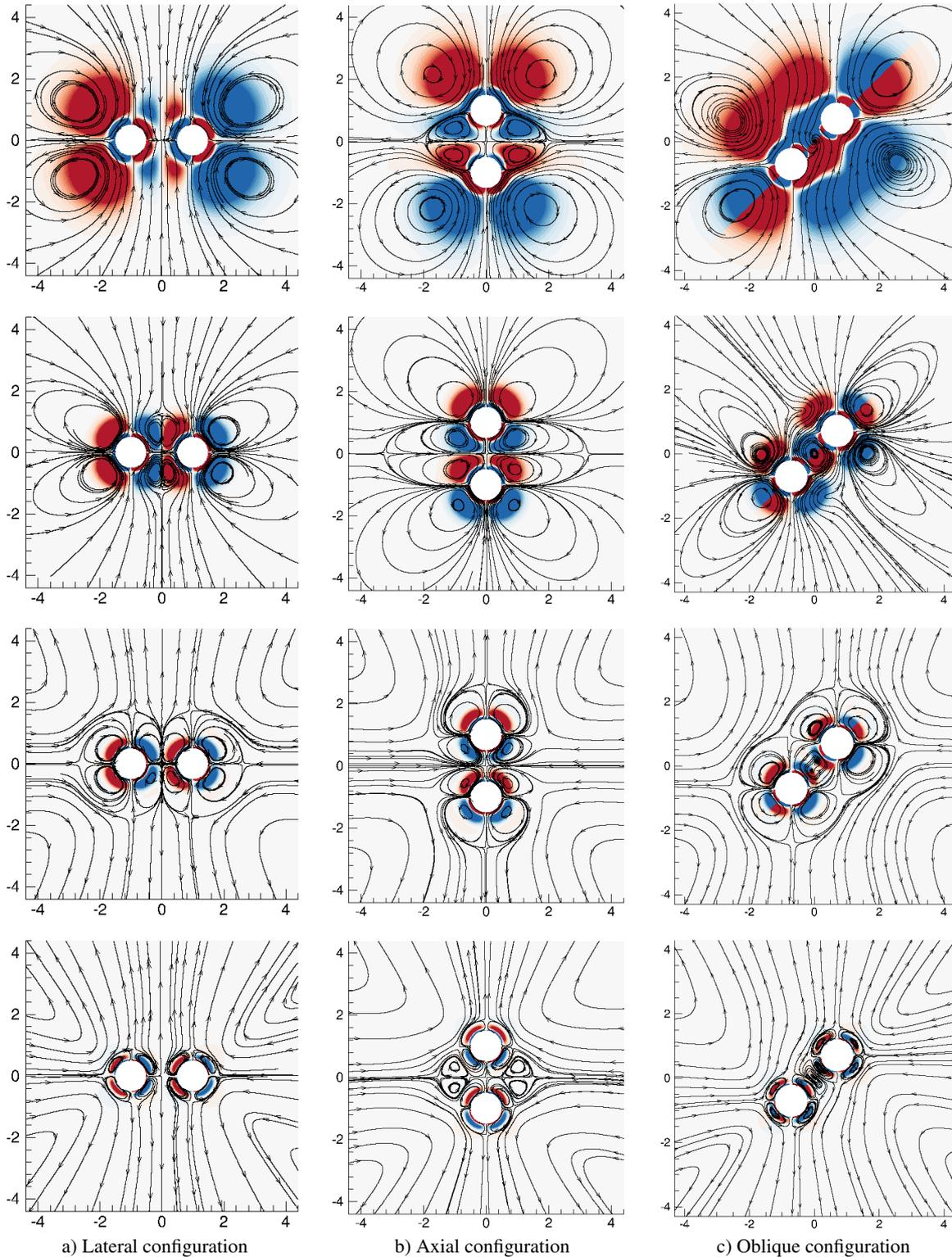
Figure 7: Steady streaming around two spheres in a) lateral, b) axial, and c) oblique configuration for  $\Omega = 1$ ,  $\Omega = 8$ ,  $\Omega = 30$ , and  $\Omega = 100$ , in each row respectively, from top to bottom, when  $L/R=2$ . The colours represent vorticity contours between  $-0.01$  to  $0.01$ .
