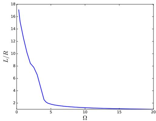
Figure 5: Distance between the center of the spheres,  $L/R$ , as a function of frequency,  $\Omega$ , in a lateral configuration.
