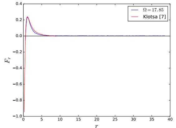
Figure 4: The curve for  $F_r$ , as a function of space between the spheres,  $r$ , using simulation by [7]. We match this curve using our simulation when  $\Omega = 17.85$ .
