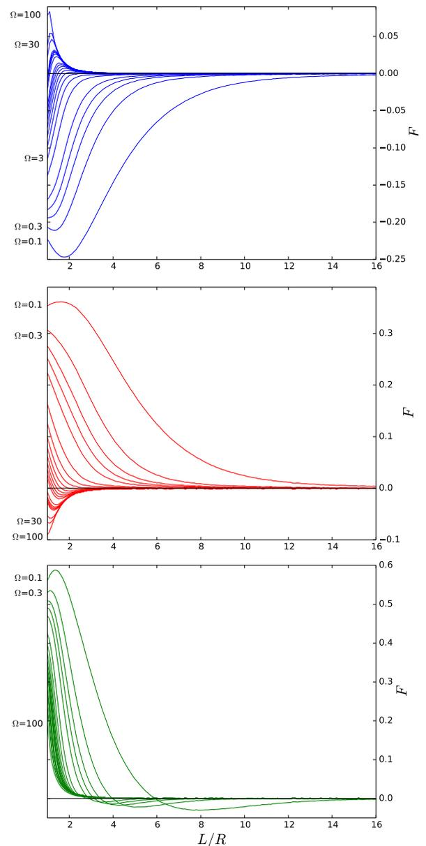
Figure 6: Non-dimensional Force,  $F$ , exerted on spheres by steady streaming as a function of distance  $L/R$  in between them for different values of  $\Omega$  in the: (a) Lateral configuration, (b) Axial configuration, and (c) Oblique configuration.
