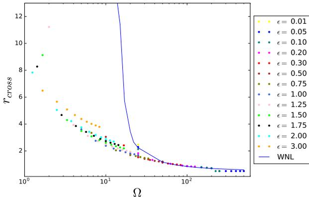
Figure 3: Comparison of size of the inner vortices,  $r_{cross}$ , in non-dimensional terms, when the oscillation of the sphere is parallel to that of the imposed oscillation, measured by DNS and WNL (using FreeFem++).
